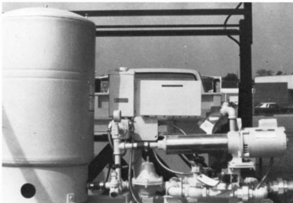
FIG. 2 Variable Speed Friction Tester Water System
