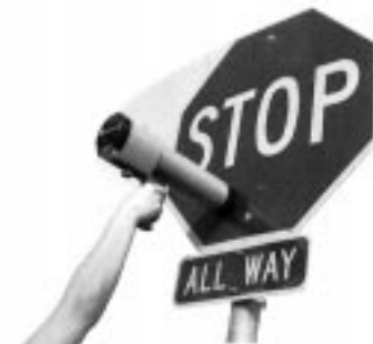
FIG. 3 Portable Retroreflectometer Positioned for Photometry of Sign Face
