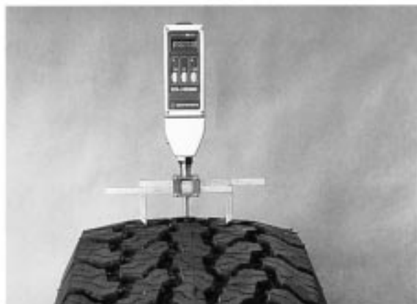
FIG. 4 Measuring the Tread Radius Using the Three Point Drop Method
