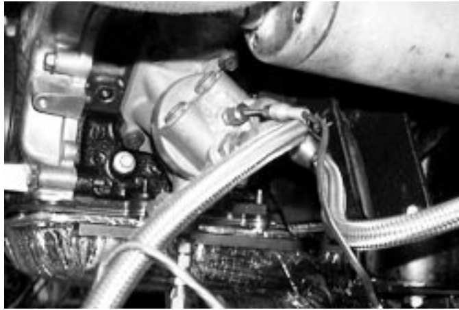
FIG. A3.25 Oil Cooling System, Adapter Housing at the Engine with Typical Fittings for Temperature Sensors, Pressure Tap and Oil Filter
