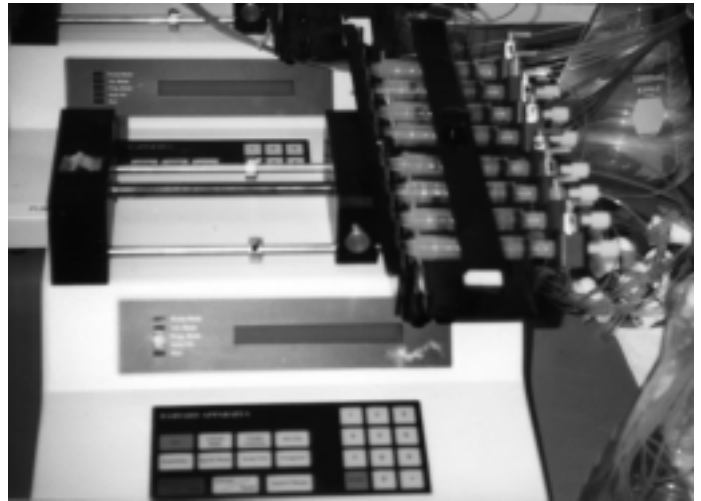
FIG. 3 Photograph of Acid Delivery System
