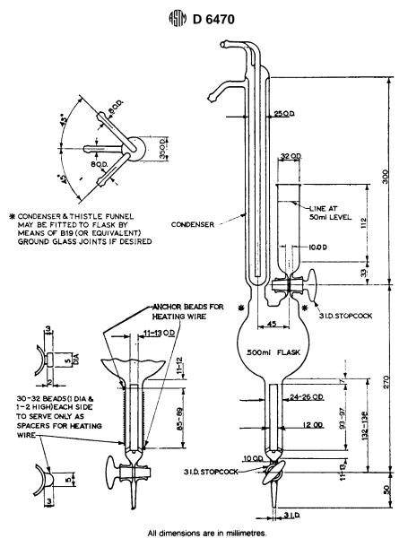
NOTE 1—Hopkins-type condenser is used. FIG. 1 Extraction Apparatus
