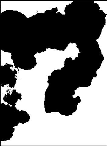
Rust Grade 1-S, 50% Rusted
