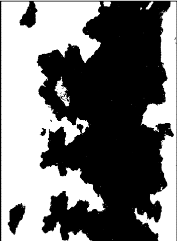
Rust Grade 1-G, 50% Rusted
