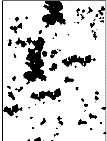
Rust Grade 3-G, 16% Rusted
