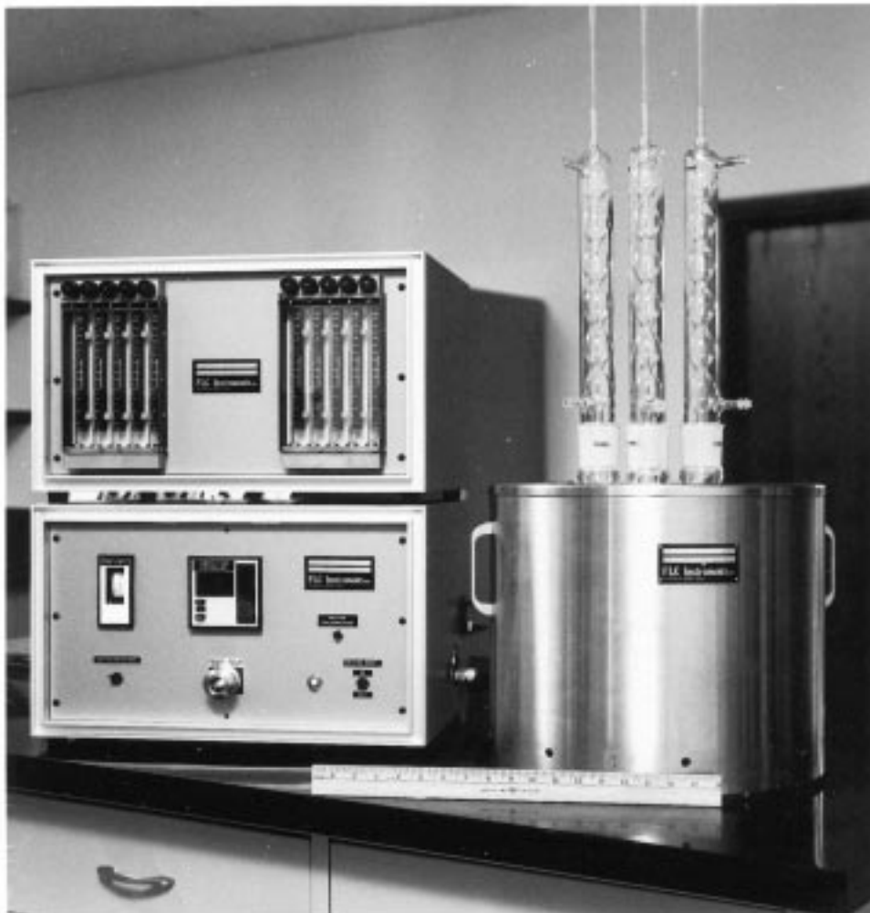
FIG. 1 Apparatus, Showing Gas Flow Control System, Temperature Control System, and Heating Block
