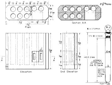
FIG. 1 Color Comparator for Carbonizable Substances in Liquid Petrolatum
