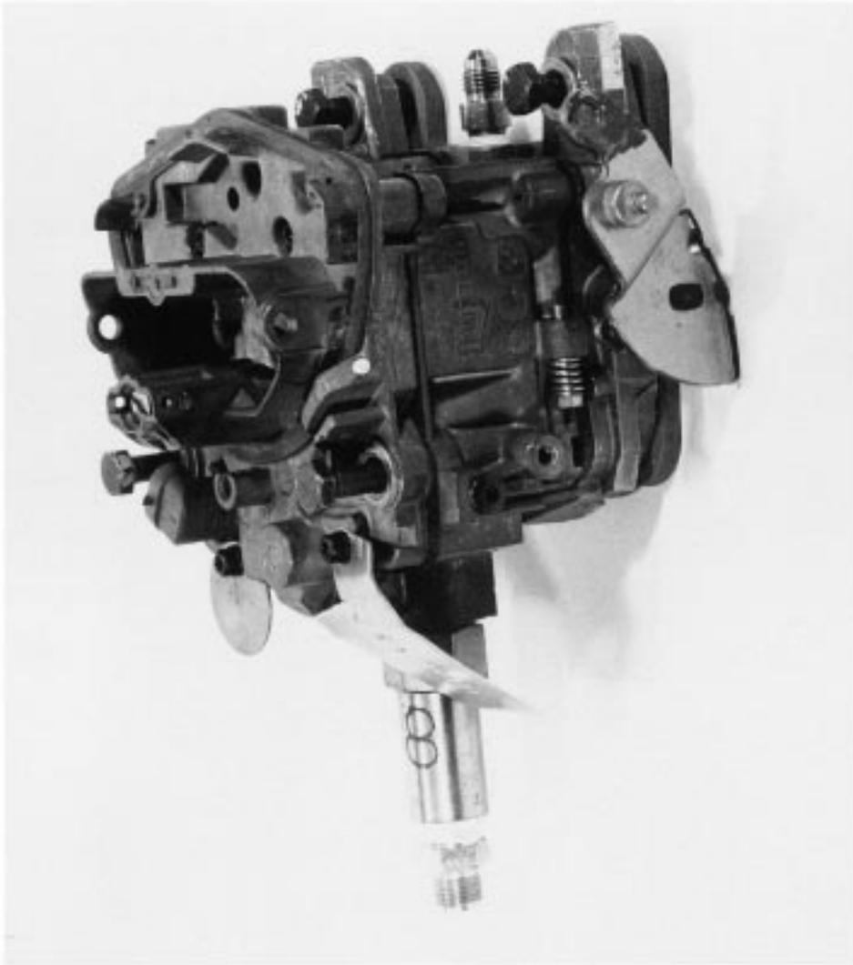
FIG. 3 Sequence III E Test Engine Carburetor
