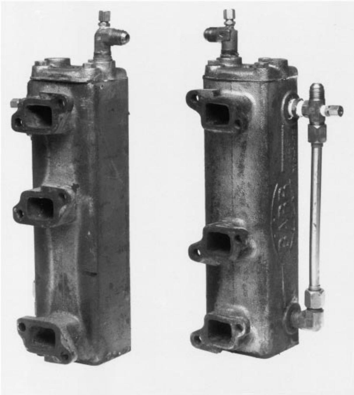
FIG. 12 Sequence IIIIE Test Engine Water-Cooled Exhaust Manifolds
