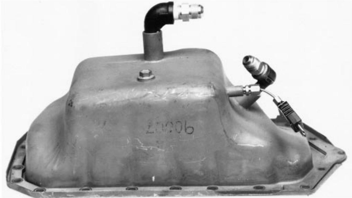
FIG. 8 Sequence III E Test Engine Oil Pan
