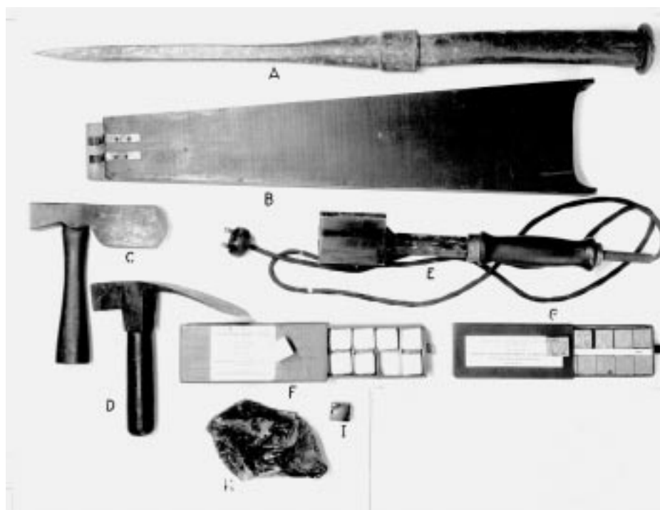
A—Rosin spike. B—Comparison box. C—Sampling hatchet. D—Sampling adz. E—Smoothing device.
