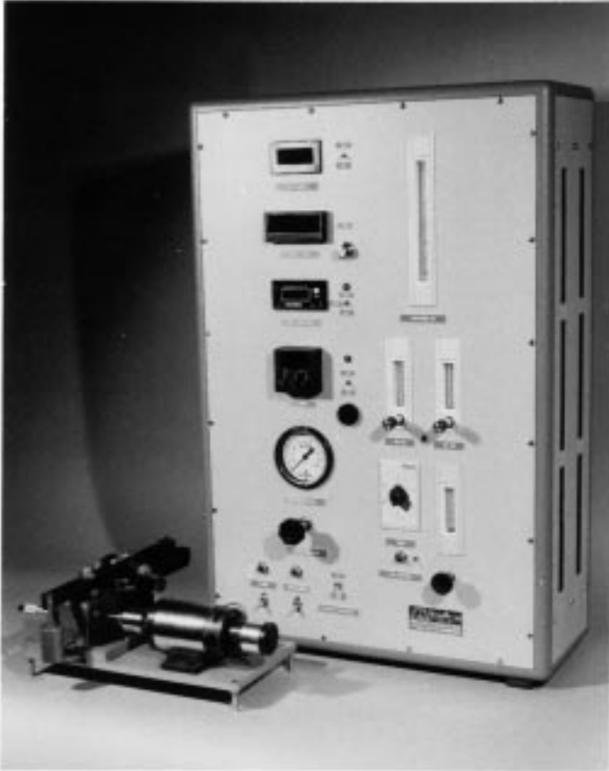
FIG. 1 Ball-on-Cylinder Lubricity Evaluator
