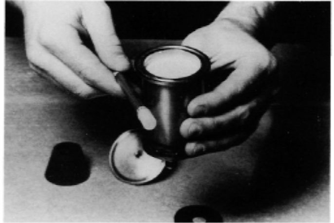
NOTE 1—Insert cone spacer, (large end of cone on top). Pour clay into cavity. Repeatedly, tap holder and add clay until level with top of cone.
