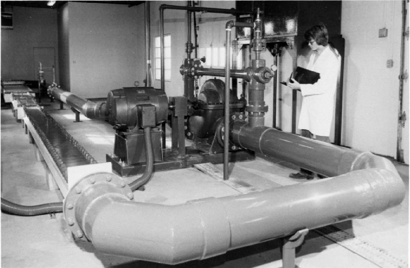
FIG. 1 High Velocity Flow Channel
