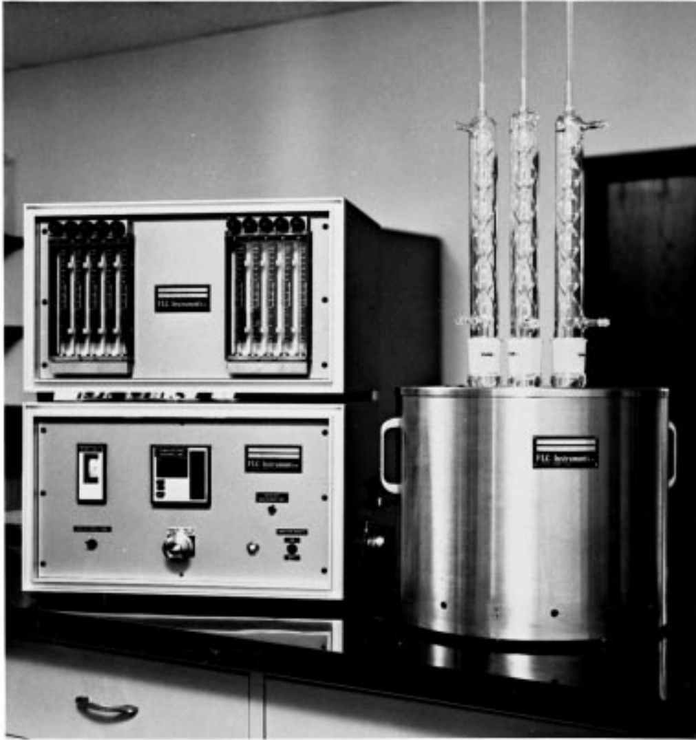
FIG. 1 Universal Oxidation Test Apparatus
