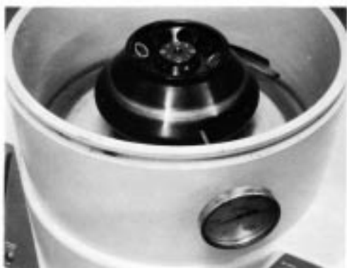
FIG. 1 Installation of Dial Thermometer (Sorvall Centrifuge)
