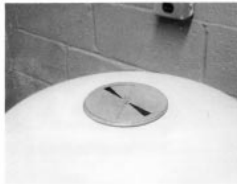
FIG. 2 Choking Air Inlet of Chamber (Sorvall Centrifuge)
