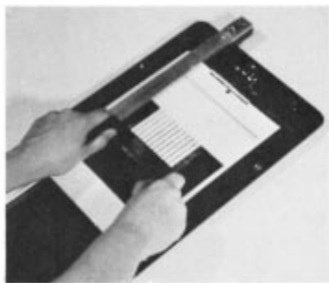
FIG. 4 Drawing Down with the Anti-Sag Meter
