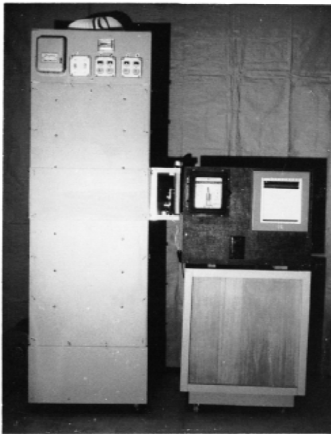
NOTE 1—Pyranometer, recorder, and demand readout meter in place. (a) Four-Bank Fluorescent Exposure Apparatus that Handles One Hundred and Eight 3 by 6-in. Panels
