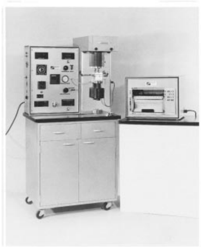
FIG. 3 Falex Variable-Speed Four-Ball Wear Test Machine
