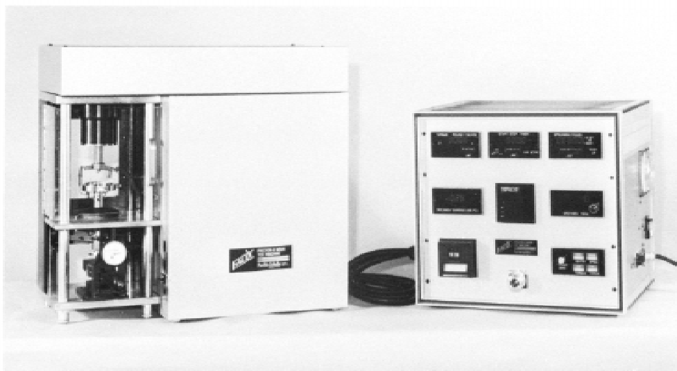
FIG. 1 The Falex Multispecimen Test Machine
